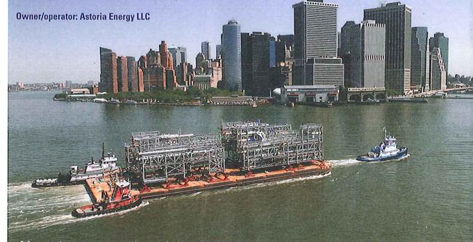
Managing construction of the 550-MW Astoria II Combined Cycle Plant in the midst of Queens, a densely packed New York City borough, required extensive off-site modular construction and a high level of logistical organization. Now the new Astoria II plant is operating successfully in conjunction with the Astoria Energy I plant as the largest natural gas—fired power plant in the Big Apple.
